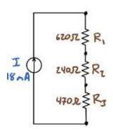
Identify two rules regarding current sources. Use these rules to determine the current through and voltage across the load resistor.
