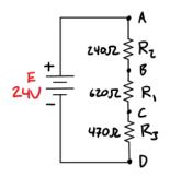
Given the above series circuit featuring rearranged elements, use Kirchhoff's Voltage Law and single subscript notation assuming node D is the reference to determine  $V_A$ ,  $V_B$ , and  $V_C$ .
