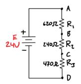
Given the above circuit use double subscript notation to identify the voltage drop across individual elements in this system.
