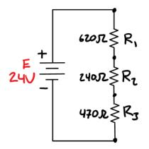
Given the above series circuit determine the total resistance, source current, and total power. Additionally, determine the voltage drop across and the power dissipated by  $R_1$  and  $R_2$ .
