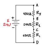
Given the above series circuit featuring rearranged elements, use Kirchhoff's Voltage Law and single subscript notation assuming node D is the reference to determine  $V_A$ ,  $V_B$ , and  $V_C$ . Discuss the implications of rearranging elements in series circuits.
