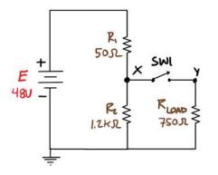
Determine the voltage across and current through each element in this system as well as  $V_{XY}$  when the switch is open and again when the switch is closed.
