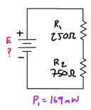
Determine the voltage drop across each element, the current through each element, the power dissipated by each element, the source current, and the total power. Additionally, determine E.
