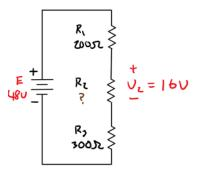
Determine the voltage drop across each element, the current through each element, the power dissipated by each element, the source current, and the total power. Additionally, determine  $V_X$ .
