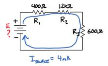
Determine the voltage drop across each element, the current through each element, the power dissipated by each element, the source current, and the total power. Additionally, determine E and R<sub>2</sub>.
