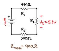
Determine the voltage drop across each element, the current through each element, the power dissipated by each element, the source current, and the total power. Additionally, determine R<sub>2</sub>.
