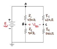
Determine the electrical properties for all elements in this system. Additionally, determine electrical properties in this system when  $R_2$  is shorted out and  $R_3$  is opened.
