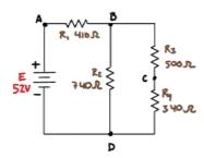
Determine the electrical properties for all elements in this system for 3 scenarios. Additionally determine the efficiency of this system given any power dissipated by  $R_X$  is considered a loss to this system.
