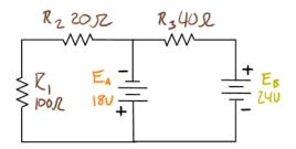
Use the superposition theorem to determine electrical properties of this circuit.
