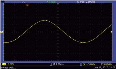
Measure the peak voltage, effective voltage, period, and frequency for this waveform given the vertical and horizontal sensitivity as displayed on the screen.
