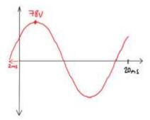
Given this plot of current as a function of time, express it in both the time and phasor domain. Draw it on a phasor diagram.
