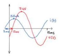
Given this phasor diagram plot voltage and current as functions of time. Determine the relative phase shift of current with respect to voltage.
