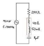
For the series AC circuit below, determine the impedance of each element, the voltage across each element, the current through each element, the total impedance, and the source current.
