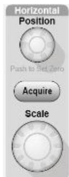
**Position.** Adjusts the horizontal position of all channel and math waveforms. The resolution of this control varies with the time base setting.
