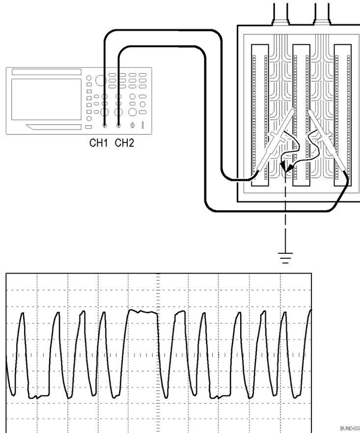
**NOTE.** Be sure to first compensate both probes. Differences in probe compensation appear as errors in the differential signal.
