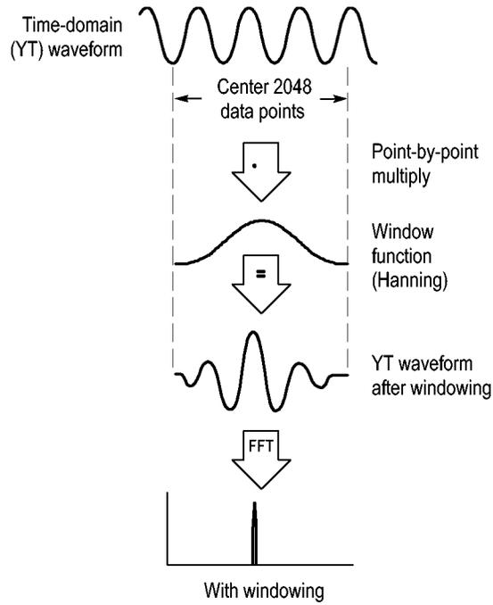
The FFT function includes three FFT Window options. There is a trade-off between frequency resolution and amplitude accuracy with each type of window. What you want to measure and your source signal characteristics will help you to determine which window to use.
