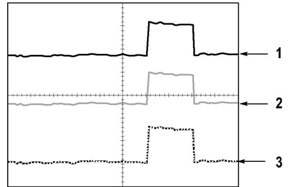
1. A solid waveform indicates a channel (live) waveform display. The waveform remains solid when the acquisition is stopped if no controls are changed that make the display accuracy uncertain.
