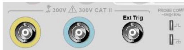
**1 and 2.** Input connectors for waveform display.
