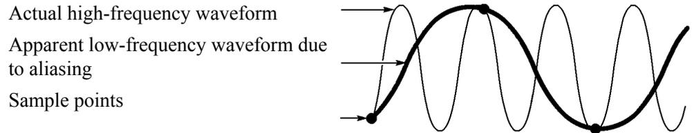
The oscilloscope accurately represents signals, but is limited by the probe bandwidth, the oscilloscope bandwidth, and the sample rate. To avoid aliasing, the oscilloscope must sample the signal more than twice as fast as the highest frequency component of the signal.
