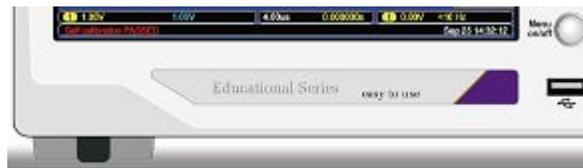
**USB Flash Drive Port.** Insert a USB flash drive for data storage or retrieval.
