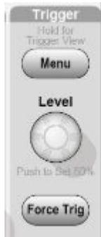
**Trigger Menu.** When it is pressed once, it displays the Trigger Menu. When it is kept pressed for more than 1.5 seconds, it will show the trigger view, meaning it will display the trigger waveform in place of the channel waveform. Use the trigger view to see how the trigger settings, such as coupling, affect the trigger signal. Releasing the button will stop the trigger view.
