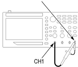
5. Push the **Autoset** button. Within a few seconds, you should see a square wave in the display of about 5 V peak-to-peak at 1 kHz.
