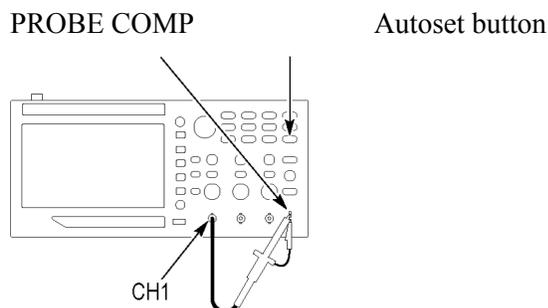
3. Check the shape of the displayed waveform.
