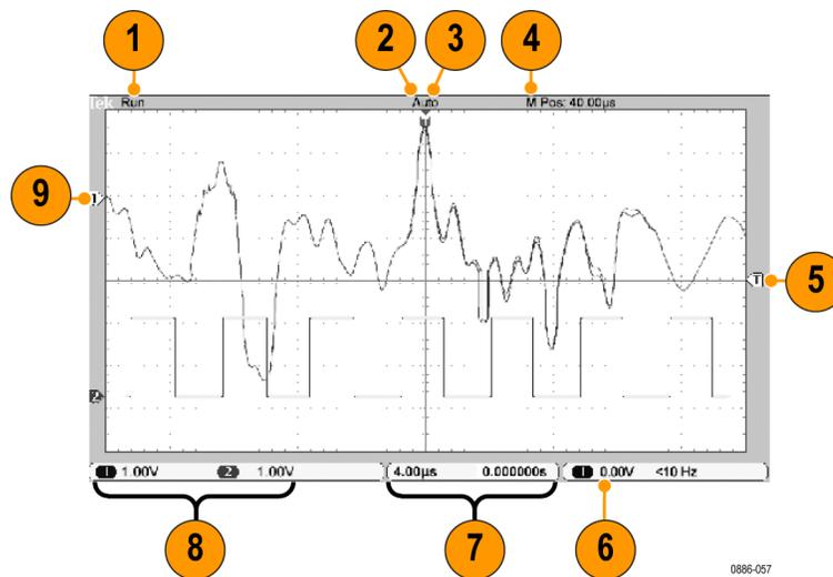
1. The acquisition readout shows when an acquisition is running or stopped.
