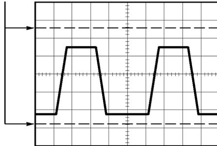
**Cursors** This method allows you to take measurements by moving the cursors, which always appear in pairs, and reading their numeric values from the display readouts. There are two types of cursors: Amplitude and Time.
