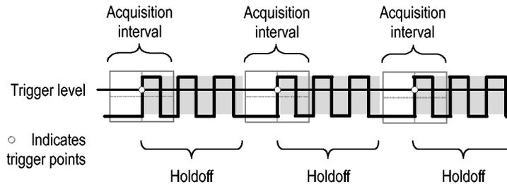
Triggers are not recognized during holdoff time.
