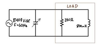
Given the above information solve for voltage, current, apparent, real, and reactive power for the load given the power factor correcting capacitor is set to 8.8uF.
