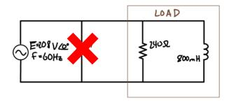
Given the above information solve for voltage, current, apparent, real, and reactive power for the load given the power factor correcting element is not in the circuit.
