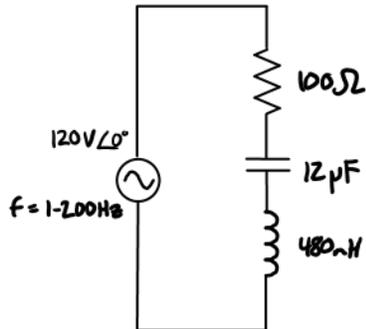
Determine the impedance for each individual element and total impedance for the series circuit above at conditions of resonance. Comment on impedance conditions at resonance.
