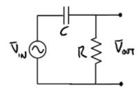
Given:  $\mathbf{V}_{IN} = 30V \angle 0^{\circ}$   $C = 0.4 \mu F$  $R = 200 \Omega$
