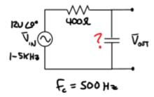
Given this series RC filter circuit determine the capacitance level necessary for a 500Hz critical frequency.
