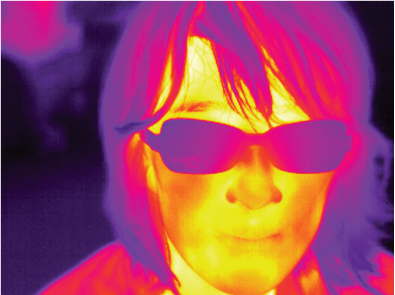
Thermograph of a person's face produced by a thermal imaging camera. The camera represents the intensity and color of detected thermal radiation that humans can't see with variations in visible color to create a false-color image. The actual light emitted by the person and detected by the thermal imaging camera has a color that we cannot see. Image Credit: "Self Portrait with Thermal Imager" by Nadya Peek via Wikimedia Commons
