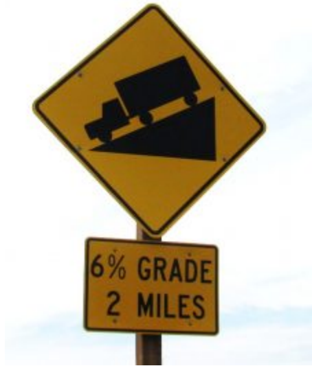
Figure 1.2. A road sign indicating a 6% grade, or 6% slope.
