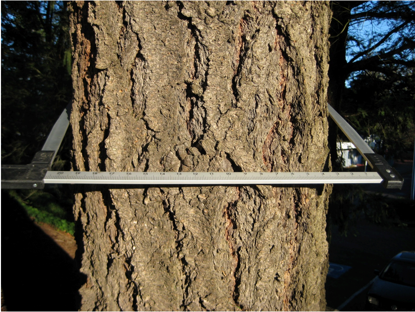
Figure 3.14. A tree caliper is held at right angles to the tree trunk. Diameter is read off the left side of the sliding scale at front.
