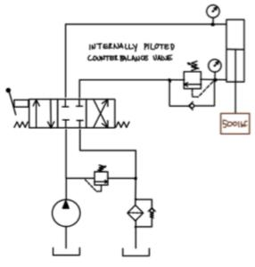
Describe the operation of this circuit making use of an externally piloted counterbalance valve used to lower a heaving mold, forming piece or platen. Comment on the behavior of this system during lowering and the maximum downwards force it is capable of generating.
