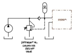
Identify the source of the differential range experienced during the operation of differential unloading relief valve
