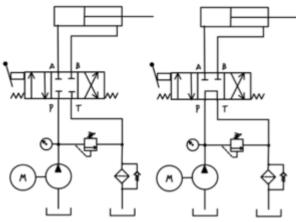
Describe why a tandem center directional control valve would not work for this circuit.
