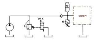
Describe how this hydraulic circuit making use of a pressure switch that turns off the prime mover when pressure is in excess of the set value contributes towards efficient operation.
