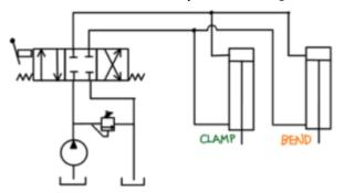
Describe the operation of this multi actuator hydraulic circuit making use of a sequence valve on the cap end of the bend cylinder. Assume the set value of the sequence valve is 400psi and the main pressure relief valve is set to 800psi.
