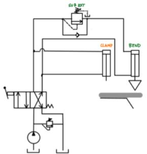
Identify potential disadvantages of coordinating actuation sequence using solely pressure input.
