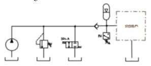
Describe how this hydraulic circuit making use of a pressure switch replicates the function of an unloading valve.
