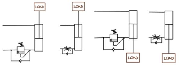
Describe the operation of this circuit making use of an internally piloted counterbalance valve. Comment on the maximum downwards force exerted by this system.
