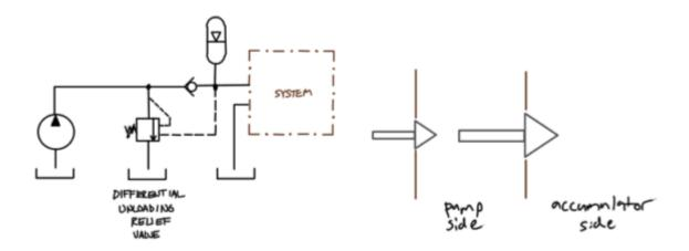
Describe the operation of this hydraulic circuit making use of a differential unloading relief valve and an accumulator.
