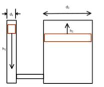
Given a force multiplication system with the following dimensions:  $d_1 = 3/4$  in  $F_1 = 120$  lbf  $h_1 = 4$  in  $d_2 = 1$  <sup>1</sup>/<sub>4</sub> in Calculate A<sub>1</sub>, p, V<sub>1</sub>, A<sub>2</sub>, F<sub>2</sub>, h<sub>2</sub>, energy<sub>in</sub>, energy<sub>out</sub>
