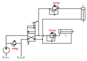
Discuss how set values of the pressure reducing valve, sequence valve, and main pressure relief valve influence the proper functionality of the above system.
