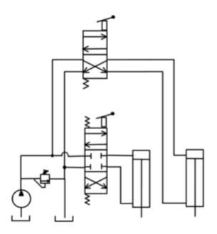
Describe the operation of this clamp and bend hydraulic circuit making use of a single directional control valve. Discuss any disadvantages of this system.
