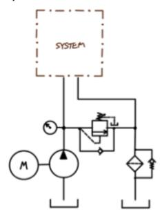
Describe how this sequence valve and check valve can be used to brake a unidirectional hydraulic motor.
