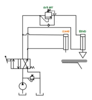
Describe the operation of this multi actuator hydraulic circuit making use of a sequence valve on the cap end of the bend cylinder and another sequence valve on the rod end of clamp cylinder.
