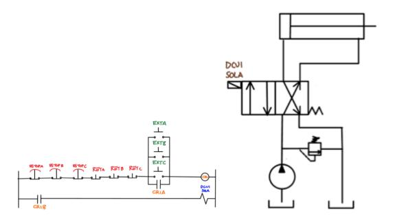
Comment on the observed behavior of a system making use of multiple push button stations if any one of the ESTOPs was accidentally triggered.
