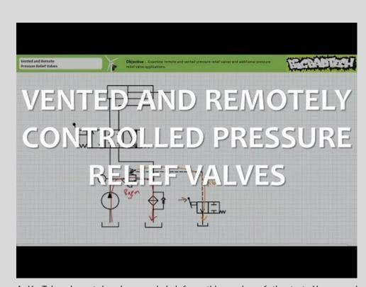
Identify pressure control valves that make use of external/remote pilot lines.
