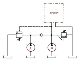
When pressure in the external pilot line reaches the set value of the unloading valve identify the magnitude of the pressure differential across the unloading valve when it opens.
