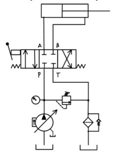
Define firing pressure. Describe why the main pressure relief valve must be above the compensator setting. Explain high pressure standby.
