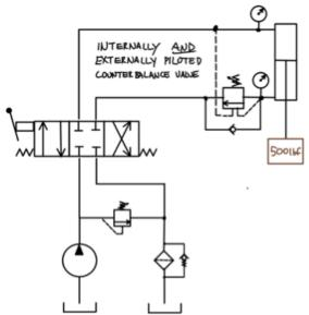
Comment on observed behavior of hydraulic systems for different counterbalance valve set values and loads.
