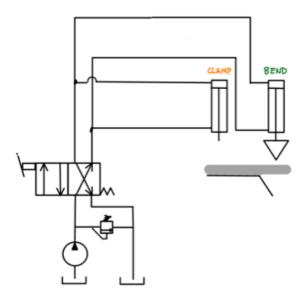
Describe the operation of this multi actuator hydraulic circuit making use of a sequence valve on the cap end of the bend cylinder. Assume the set value of the sequence valve is 400psi and the main pressure relief valve is set to 800psi.
