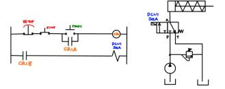
Describe the behavior of this electrically controlled hydraulic system incorporating a limit switch.
