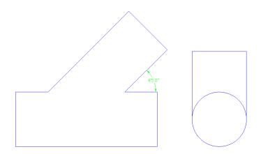
Now as before, we will draw half circle on the ends of pipe and divide them up into equal parts to help develop our element lines. Remember to number the lines as well so when we draw out the stretch-out.
