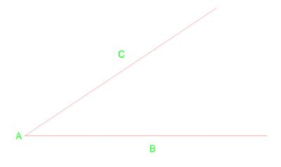
First we can draw an arc from vertex A that crosses the line near point C & B. From those two intersection we can then draw two additional arcs to the right.
