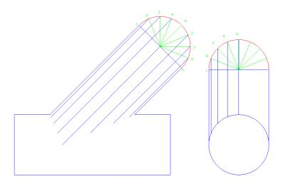
Now we can draw lines horizontally between the two views to help develop the first set of lines we will need. Line up and draw from point 1 to point 1 and so on through point 5. You will notice how the lines will go straight through line 6, 7, 8 & 9. Since this is a concentric reducer from end view, the points will be the same on both side of the pipe. Place a tick mark and each point of intersection.
