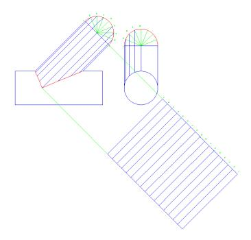
Now we can transfer lines at a 45° angle down from the side view and connect them to same number lines on the stretch-out. Place a tick mark on each point that intersect with the same number as that of where the line originated from.
