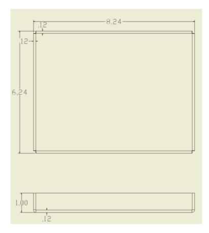
The outside dimension are 6.24" x 8.24" x 1" tall. To figure out what inside dimension is for bottom of pan for layout we need to take 2 x the sheet thickness minus the given outside dimension. The inside dimension of pan is 6" x 8" with an inside height of .88".
