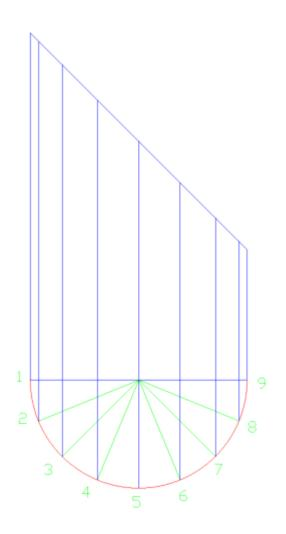
Now we will construct the stretch out of the template. Extend the bottom and top lines to the right from the first view drawn. The overall length of your stretch out will be determined by the circumference of your pipe. The green line indicate how we transfer the overall height of object to the stretch-out.
