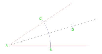
Using this method will equally split the angle into two angle of the same measurement. This method and can repeated if necessary to split it again into 4 equal parts.
