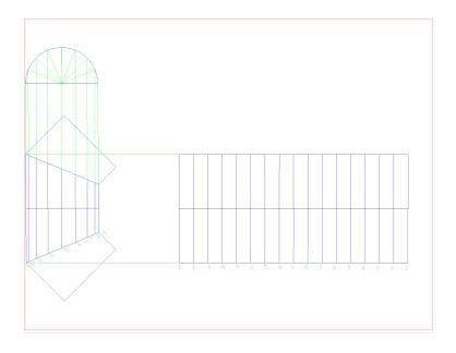
Now we can transfer elements to the stretch-out. Indicated by dashed lines you see how they reference the numbered lines on each drawing.
