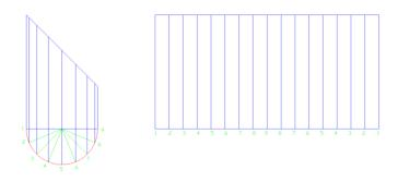
The numbers will correlate to each other from one drawing to the other. Place a straight horizontal line from mitered line over to the stretch-out and where the numbers math-up, make a tick mark.
