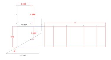
Next we will transfer the measurements from the side view to the stretch-out to determine the shape of the template.
