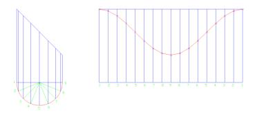
You can now remove the top section of lines above the curve on the stretch-out. Cut your template out and it is ready to use.
