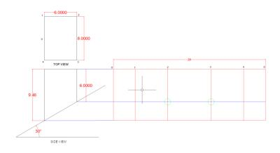
Now we can add a couple lines connecting the base of the stretchout to vertical line 2 & 3 to show what the final shape of stretch-out will be. We can also remove any lines we used to transfer features from side view to stretch-out. The green line indicate the sheet size and shape the red lines indicate where the sheet will be formed.
