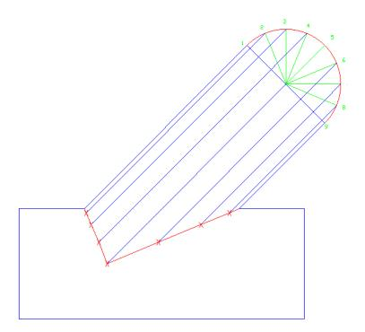
Now we can make our stretch-out from the 45 lateral and divide up as we have on past templates. Divide the stretch-out up into 160 equal spaces.
