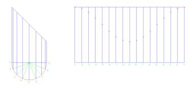
Now with connect a line between tick marks with a curved line.
