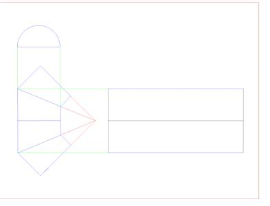
Next we will divide the half circle into 8 equal parts and the stretchout into 16.
