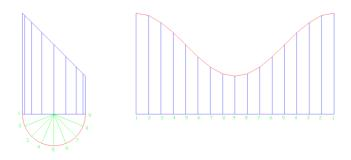
Now you can take the stretch-out and wrap around your pipe, trace the curved line onto pipe and proceed to cut.
