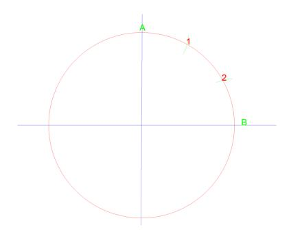
By setting your compass to the radius of the circle, 1 <sup>1</sup>/<sub>2</sub>" and then drawing an arc from point A and then B they intersect at 1 & 2. If you then to draw a line from the center of the circle to each point, you just divided that quarter of the circle into three equal parts. See below...
