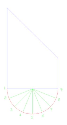
Now, at each point on the arc draw a straight line from arc to where it intercepts the  $45^{\circ}$  line. Those are you element lines.
