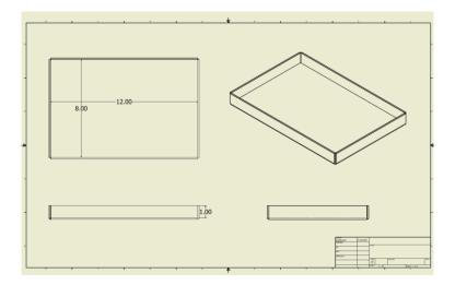
Now that we have the parts overall size we can determine how to go about laying this part flat and work with the dimensions given so we can create the pan.
