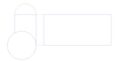
Now we can divide up the stretch-out into 16 equal spaces and divide the half circle up as well. Note: Since this is an eccentric branch and it is not on center. We have to divide up the entire half circle.
