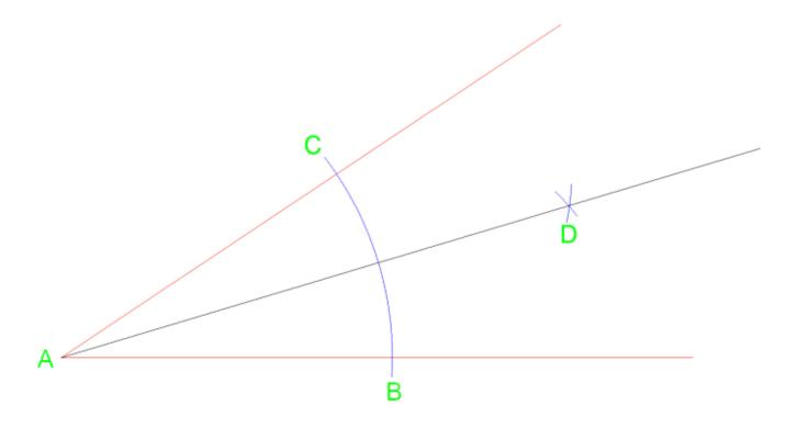
Using this method will equally split the angle into two angle of the same measurement. This method and can repeated if necessary to split it again into 4 equal parts.
