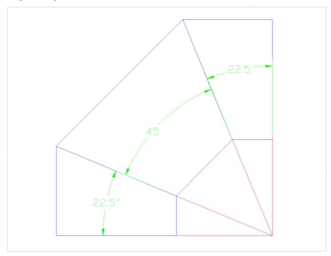
When will use the center portion of our elbow to make our stretch-out and begin to develop the template.
