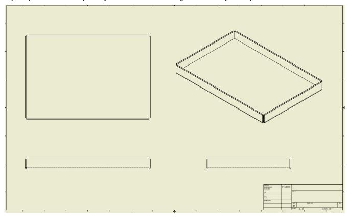
Here we have both the perspective view and an orthographic drawing. Using this format it is easy to see what the finish product will look like. What we have to do here is reverse the process to see what shape we have to start with to build the pan. The one thing we need now are dimensions.
