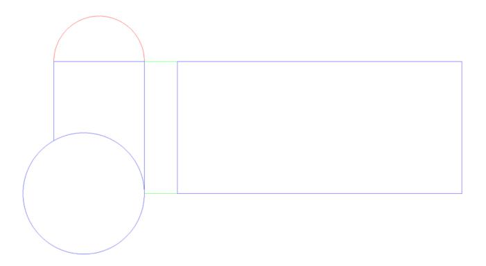
Now we can divide up the stretch-out into 16 equal spaces and divide the half circle up as well. Note: Since this is an eccentric branch and it is not on center. We have to divide up the entire half circle.
