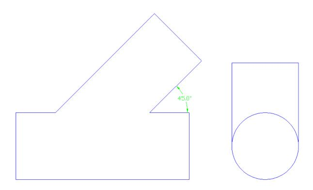
Now as before, we will draw half circle on the ends of pipe and divide them up into equal parts to help develop our element lines. Remember to number the lines as well so when we draw out the stretch-out.
