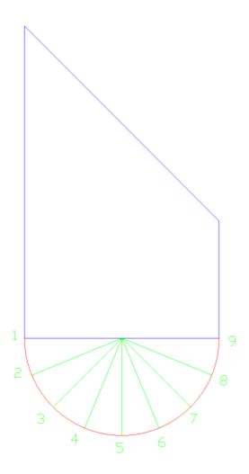
Now, at each point on the arc draw a straight line from arc to where it intercepts the 45° line. Those are you element lines.
