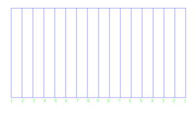
The numbers will correlate to each other from one drawing to the other. Place a straight horizontal line from mitered line over to the stretch-out and where the numbers math-up, make a tick mark.
