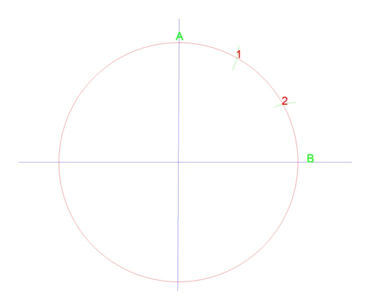
By setting your compass to the radius of the circle,  $1\frac{1}{2}$ " and then drawing an arc from point A and then B they intersect at 1 & 2. If you then to draw a line from the center of the circle to each point, you just divided that quarter of the circle into three equal parts. See below...
