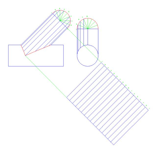
Now we can transfer lines at a  $45^{\circ}$  angle down from the side view and connect them to same number lines on the stretch-out. Place a tick mark on each point that intersect with the same number as that of where the line originated from.
