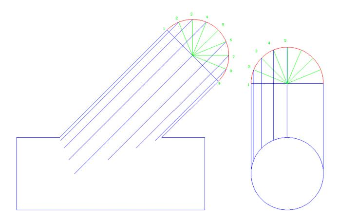
Now we can draw lines horizontally between the two views to help develop the first set of lines we will need. Line up and draw from point 1 to point 1 and so on through point 5. You will notice how the lines will go straight through line 6, 7, 8 & 9. Since this is a concentric reducer from end view, the points will be the same on both side of the pipe. Place a tick mark and each point of intersection.
