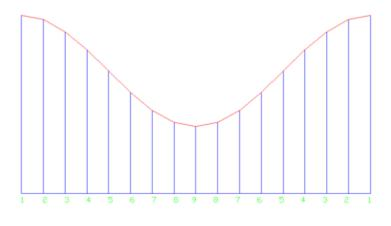
Now you can take the stretch-out and wrap around your pipe, trace the curved line onto pipe and proceed to cut.
