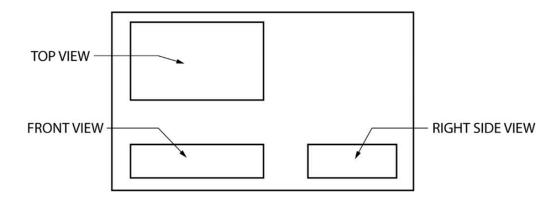
There will be times when you will have to in vision either the perspective view or the orthographic drawings to help you through the build process. It is sometimes helpful to make even a hand sketch of the missing drawing to help you see what is being built.
