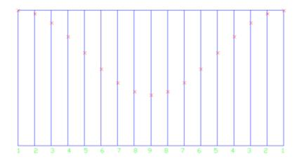
Now with connect a line between tick marks with a curved line.
