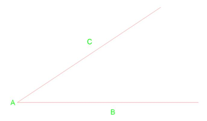
First we can draw an arc from vertex A that crosses the line near point C & B. From those two intersection we can then draw two additional arcs to the right.
