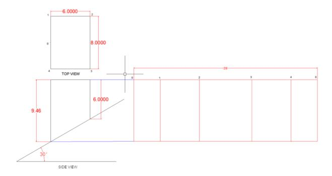
Next we will transfer the measurements from the side view to the stretch-out to determine the shape of the template.
