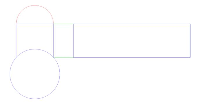
Now we can divide up the stretch-out into 16 equal spaces and divide the half circle up as well. Note: Since this is a concentric branch and everything is off of center, we can get away with only dividing half the half circle, it is a mirror of the other side.
