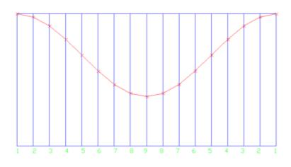
You can now remove the top section of lines above the curve on the stretch-out. Cut your template out and it is ready to use.
