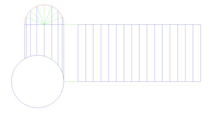
Now we can transfer lines from end view to the stretch-out and number match them and place out tick marks. Remember to number each line as well.
