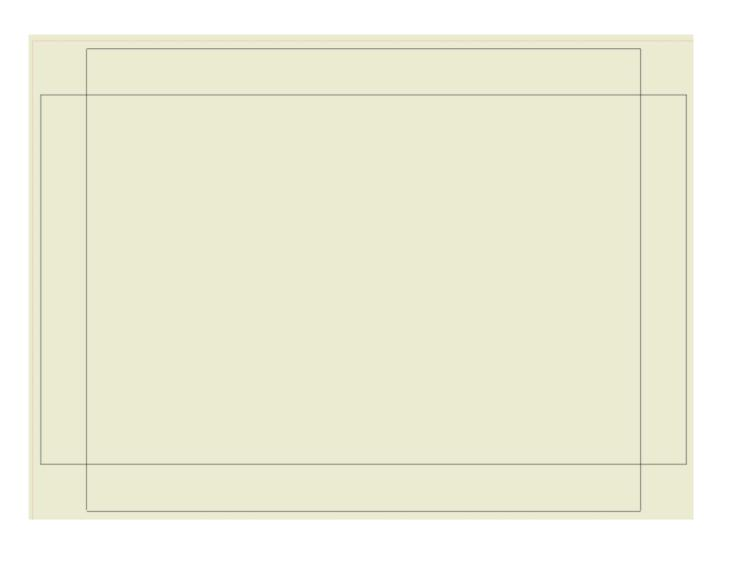
Now you can see in each corner there is a square notch. These notches allow 1" portion of the sheet to be bent up  $90^{\circ}$ to form the pan.
