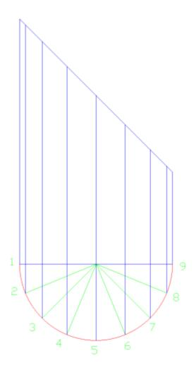
Now we will construct the stretch out of the template. Extend the bottom and top lines to the right from the first view drawn. The overall length of your stretch out will be determined by the circumference of your pipe. The green line indicate how we transfer the overall height of object to the stretch-out.
