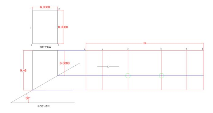
Now we can add a couple lines connecting the base of the stretch-out to vertical line 2 & 3 to show what the final shape of stretch-out will be. We can also remove any lines we used to transfer features from side view to stretch-out. The green line indicate the sheet size and shape the red lines indicate where the sheet will be formed.
