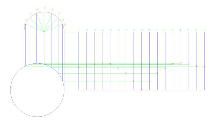
Now we can draw our curved line between tick marks and remove transfer lines.
