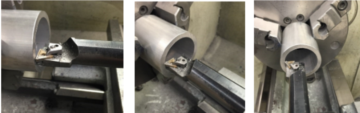
Figure 4. Boring on a lathe
