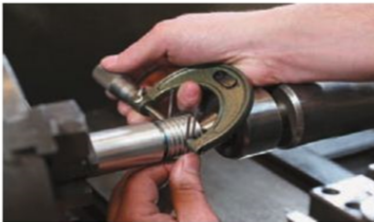
Figure 16. Three wire measurement
