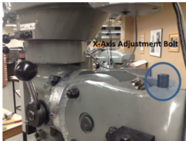
Adjustment bolt used to position the mill head vertically around the X-axis.
