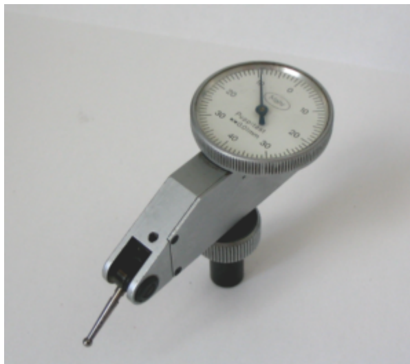
Dial indicator used for tramming the head.
