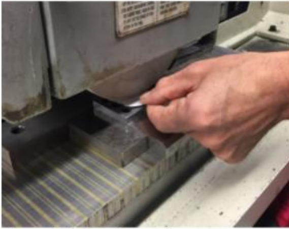
Figure 6. Setting the z axis
