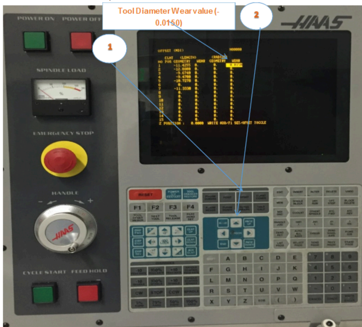
Figure 20. Adjusting CDC Offsets
