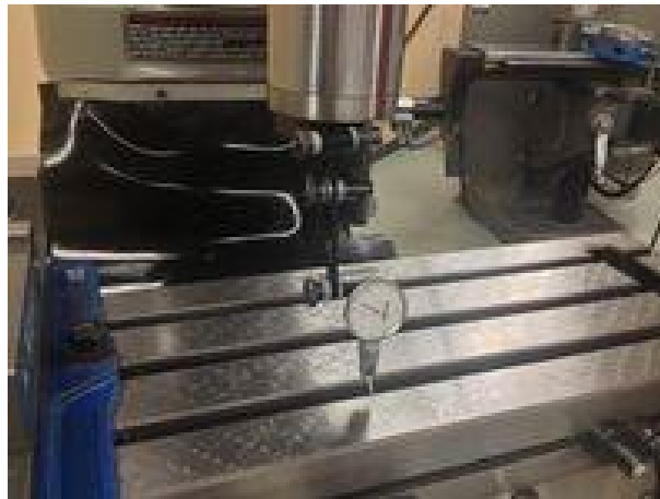
Dial indicating around the mill head X-axis.
