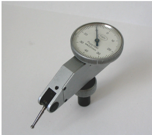
Dial indicator used for tramming the head.
