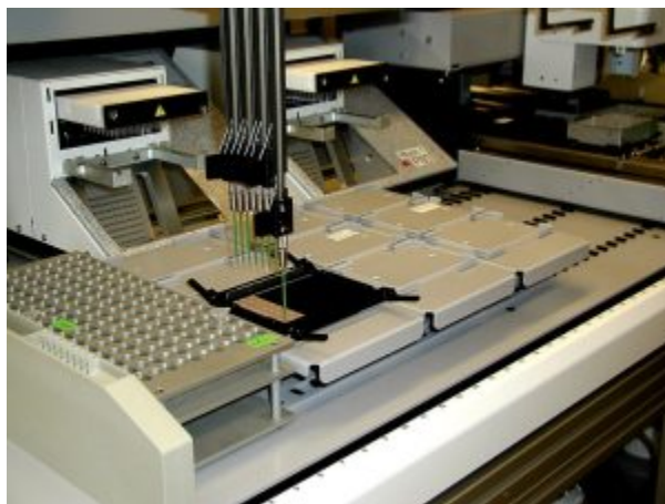
Figure 1: This machine is preparing to do a proteomic pattern analysis to identify specific cancers so that an accurate cancer prognosis can be made. (credit: Dorie Hightower, NCI, NIH)
