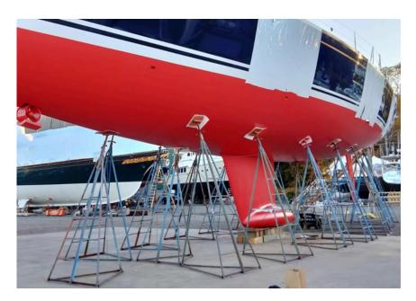
Triangular supports hold a boat in the air while it undergoes repairs at the Front Street Shipyard in Belfast, Maine.
