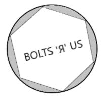
7. The hexagonal head of a bolt fits snugly into a circular cap with a circular hole with inside diameter  $46~\mathrm{mm}$  as shown in this diagram. Opposite sides of the bolt head are  $40~\mathrm{mm}$  apart. Find the total empty area in the hole around the edges of the bolt head.
